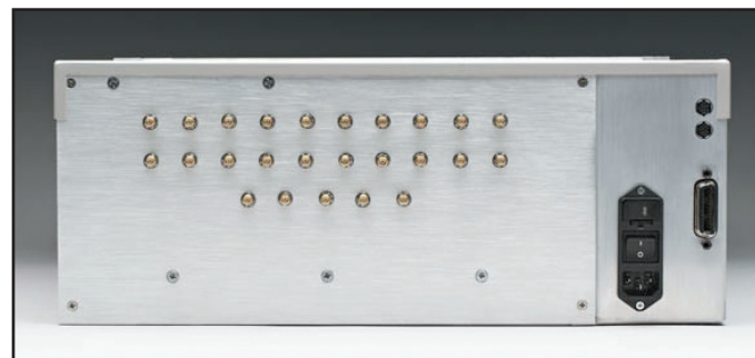
Rear panel bulkhead connectors
